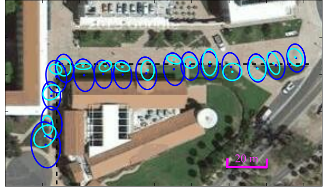
Fig. 10. The resulting geo-location improvement from Algorithm 3. The blue ellipses represent geo-location reported by the GNSS receiver. The cyan ellipses represent the geo-location resulting from using the map matching algorithm. The black dashed line represents ground truth of the GNSS receiver trajectory.
