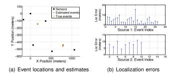
Fig. 4. Results of the multiple event localization algorithm. The true and estimated event locations are shown on the left and the localization errors are shown on the right.
