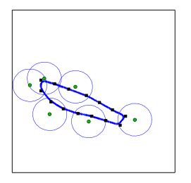
Fig. 5. Path taken by mule-UAV during tests. The desired path was sent to autopilot via square waypoints. The sensors and communication regions are represented by green and blue circles respectively.
