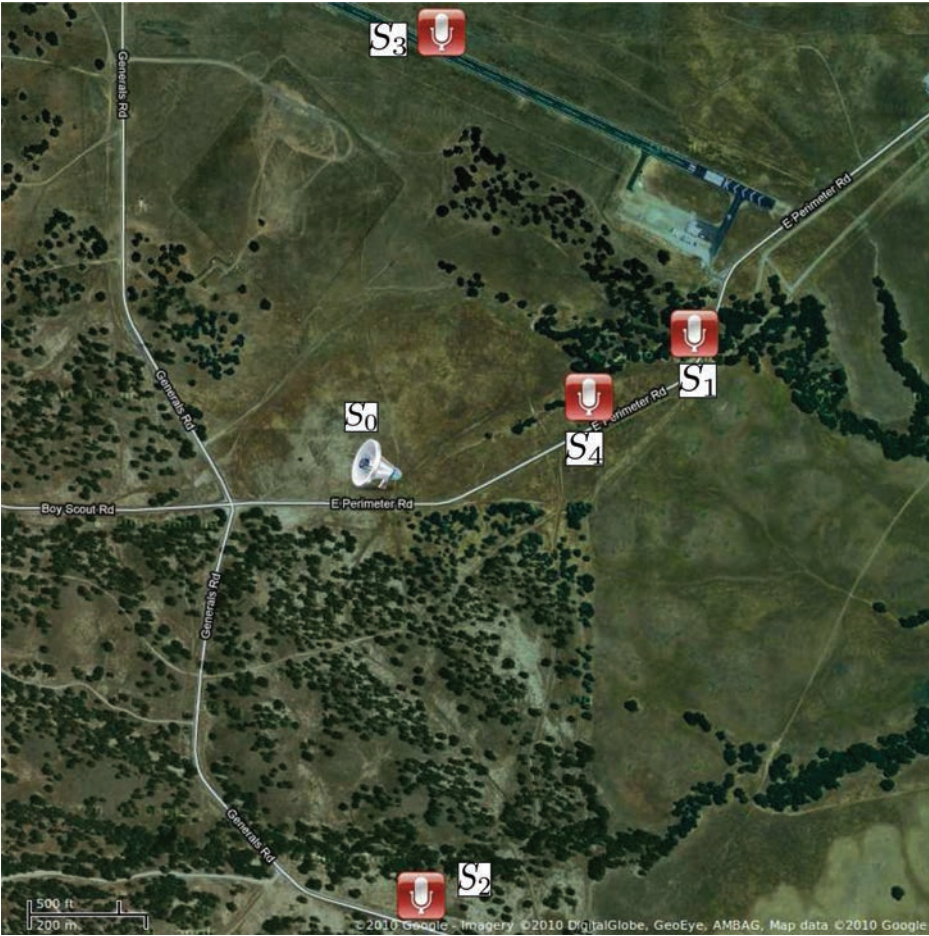
Fig. 8. Sensor configuration for January 28, 2010 morning tests. In the afternoon tests, the location of sensor 4 was switched with the position of the acoustic source.
