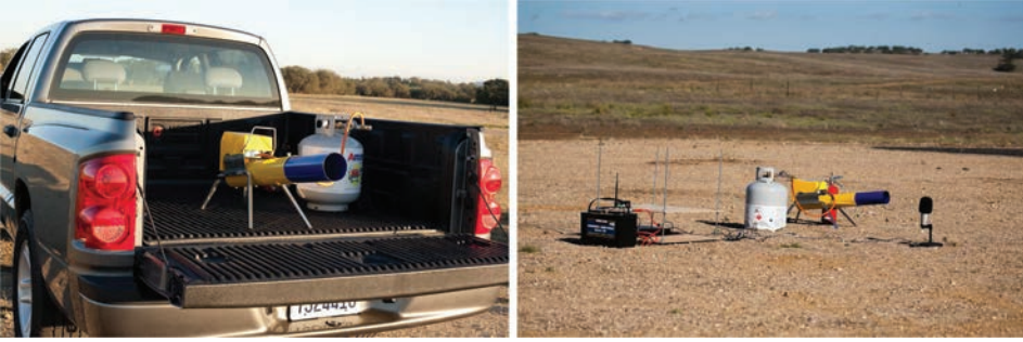
Fig. 4. The propane cannon used to create acoustic disturbances.
