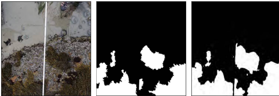
Figure 26: Result of unprocessed test image. The left image is original image, center image is the annotated image, right image is the predicted mask.
