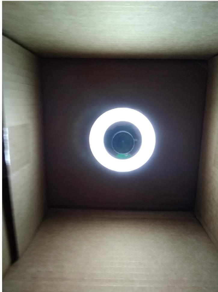
Figure 12: How the camera lens is positioned within the LED ring light.
