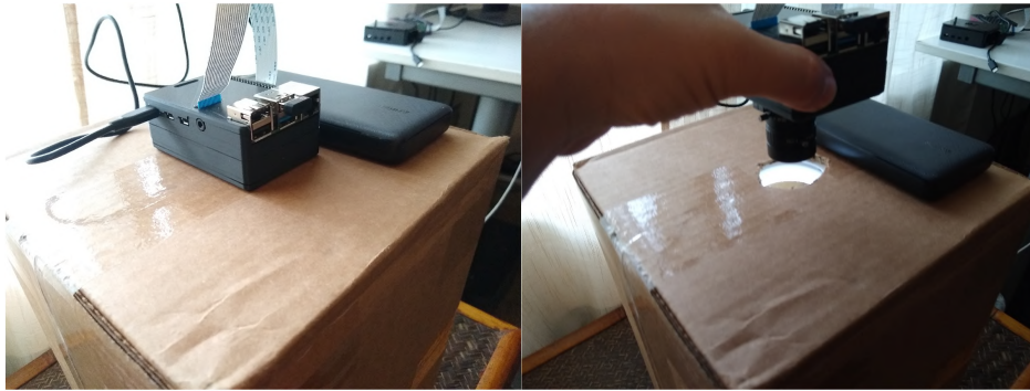
Figure 10: Raspberry Pi High Quality Camera with Arducam 8mm lens, on top of robot prototype, along with a power bank.
