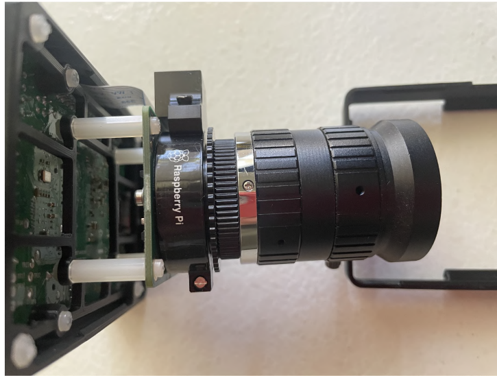
Figure 6: Raspberry Pi High Quality Camera with lens, attached to Raspberry Pi 4.
